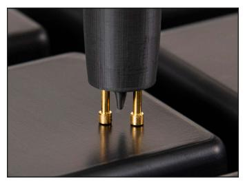
Figure 2. Orienting the spring-loaded pins onto the material to be tested
