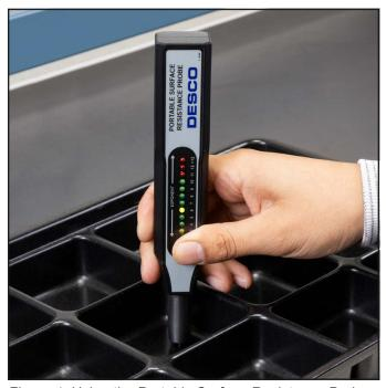
Figure 4. Using the Portable Surface Resistance Probe
