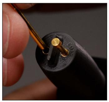
Figure 5. Replacing the spring-loaded pins
